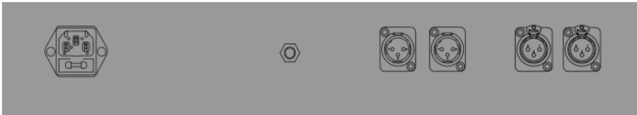
**Input:** Signal input for left and right channels
