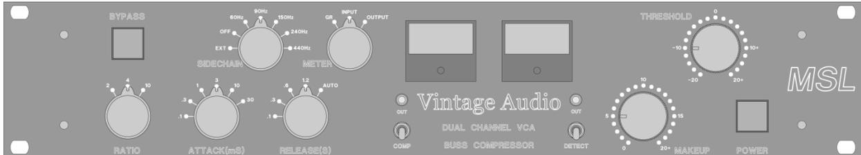
**True Bypass:** The MSL features a true relay bypass that effectively routes the input to the output bypassing the circuit completely. This is a nice feature when you simply need an accurate reference.
