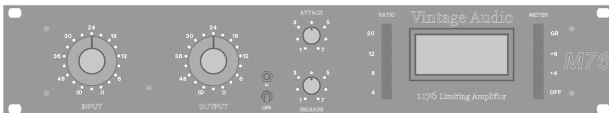
**Input Control:** Here the user is able to adjust the amount of input level sent into the M76's internal circuitry. The input level attenuator determines how much of the signal is over the threshold and therefore compressed.
