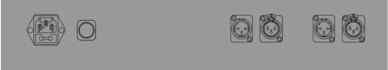
**Input:** Signal input for channel one and channel two respectively. Microphone as well as line signals can be inputted into the M73. When using line level signals make sure to have the 20 db pad engaged.
